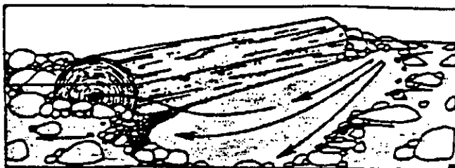
Figure 10. Lateral scour pool associated with large debris.
