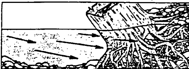
Figure 11. Lateral scour pool associated with rootwad.
